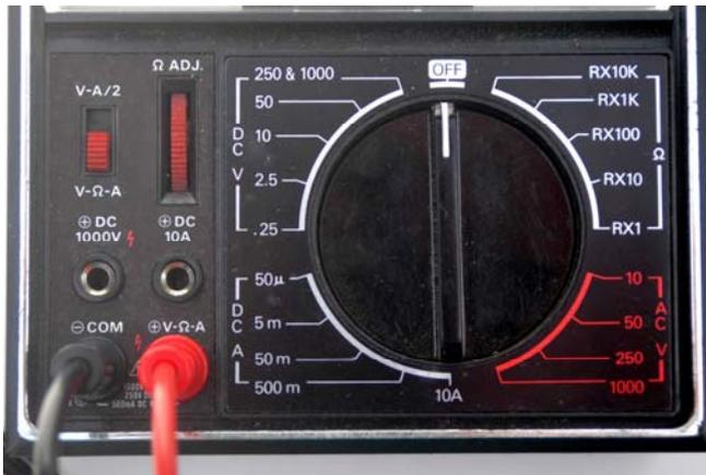
This is the dial for the analog multi-meter. Note the DC volts scale at the upper left. When looking for voltage on our cars we would use the 50 volt scale since that is the next scale *higher* than our 12 volts.
