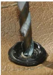
I used a 3/8 inch bit to remove enough metal to separate the top and bottom of the snap. Take your time here and grind away just enough to do the job.
