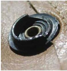
Many of us have convertible top boots and tonneau covers with plastic snaps. After years of use, the plastic becomes brittle and breaks as shown in the illustration to the left. In this article I will show you how to remove the broken snaps and install a new metal one that will last as long as the car does.
