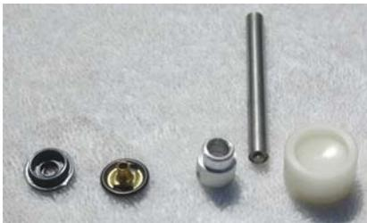
The parts for replacement as shown here are, from left to right, socket, button, guide tool, flaring tool, and anvil. The first order of business is to remove the broken snap. I have found the best way to do this is with a drill. Choose a bit that will cover the center part of the underside of the button. Use it on a sacrificial piece of lumber, not the kitchen table.
