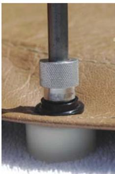
Use a hammer to tap the flare tool on the end several times to "brad" the two pieces of the snap together. The snap will now be repaired and will be good for years of use as shown to the right.
