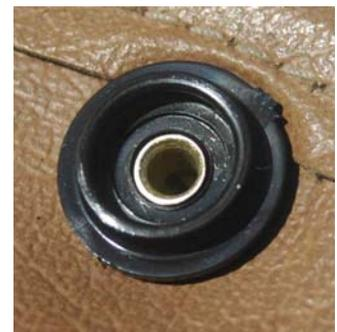
Total time: 15 minutes, or less. I prefer to use the kits with the anvil. Some kits eliminate the guide by making the flaring tool the same size and the inner diameter of the snap
