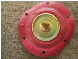
Since I'm getting very good at removing the pump, I determined the problem in about 5 minutes. The diaphragm was flaking apart and kinda gooey. It finally dawned on me that I was suffering from the same thing as all those boaters with melting fiberglass gas tanks....Ethanol!
