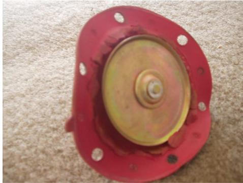
check valve was swelled and was no longer keeping the gas moving on one direction towards the Carburetors.
