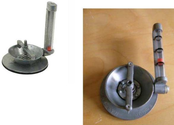
After loosening the linkages that interconnect the two carburetors and removing the air filters, the Uni-Syn is held momentarily over the throat of each carburetor. The air passing through the device causes a little red indicator to rise up in the tube. The more air that passes through the device, the higher the indicator rises in the tube. To balance the carburetors, adjust the idle screws so that the indicator rises to the same point when held over the throat of each carburetor.
