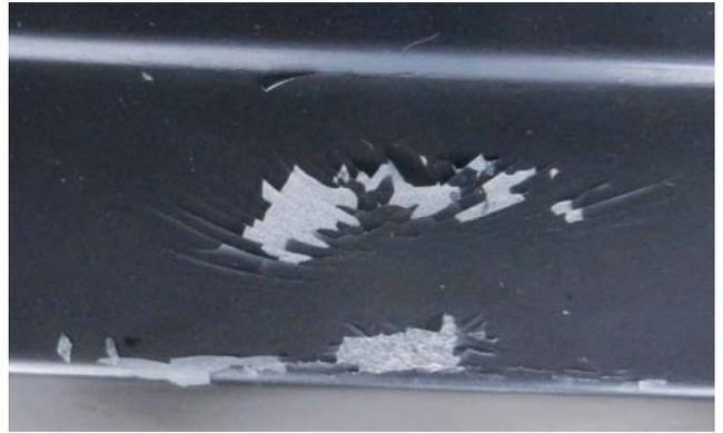
My first inclination was to mask off the painted areas of the car behind the bumper and do all the work with the bumper still mounted. Masking would make sure that I did not accidentally sand into the painted surface of the car. After working this way for an afternoon I decided to do the job right I would need to remove the bumper and work on a workbench. I removed the bumper and put a drop cloth over my Work Mate and laid the bumper over it.
