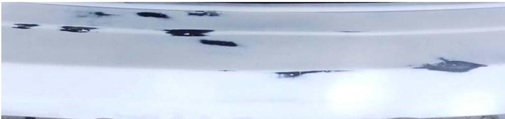
About an hour before spraying I used **Prep All® Wax and Grease Remover** as a final step to prepare the surface. It dries fairly fast, just make sure there is none left on the surface.
